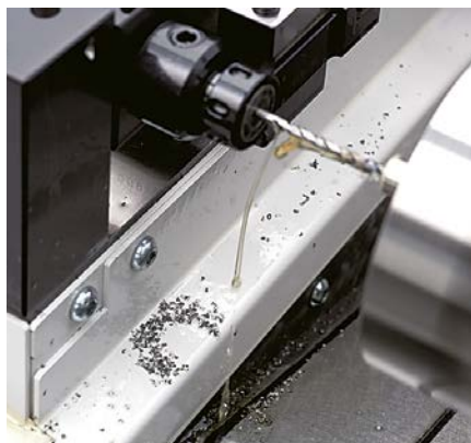
Deep hole drilling utilising oil hole drills. Broken chips are discharged up through the flutes on the drill, which prevents entanglement.
