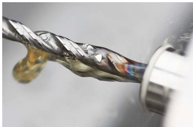
Chips generated by LFV
