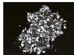
Chips generated by LFV
